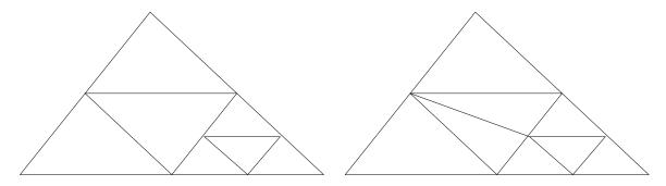
FIGURE 1. Red refinement of a triangle (left) resulting in a hanging node, and green refinement (right) to enforce compatibility.
