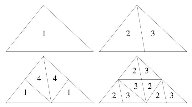
FIGURE 2. Three levels of newest vertex bisection showing the four similarity classes of resulting triangles.
