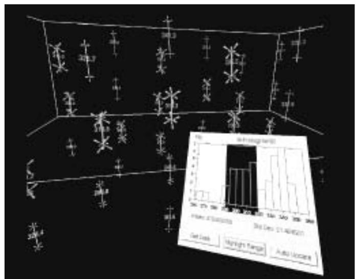
**Figure 4.** Selected histogram bins are highlighted in visualization showing distribution of strut diameters in the range of 200 to 320  $\mu\text{m}$ . The struts have been removed from the scene in order to make the measurements more visible.
