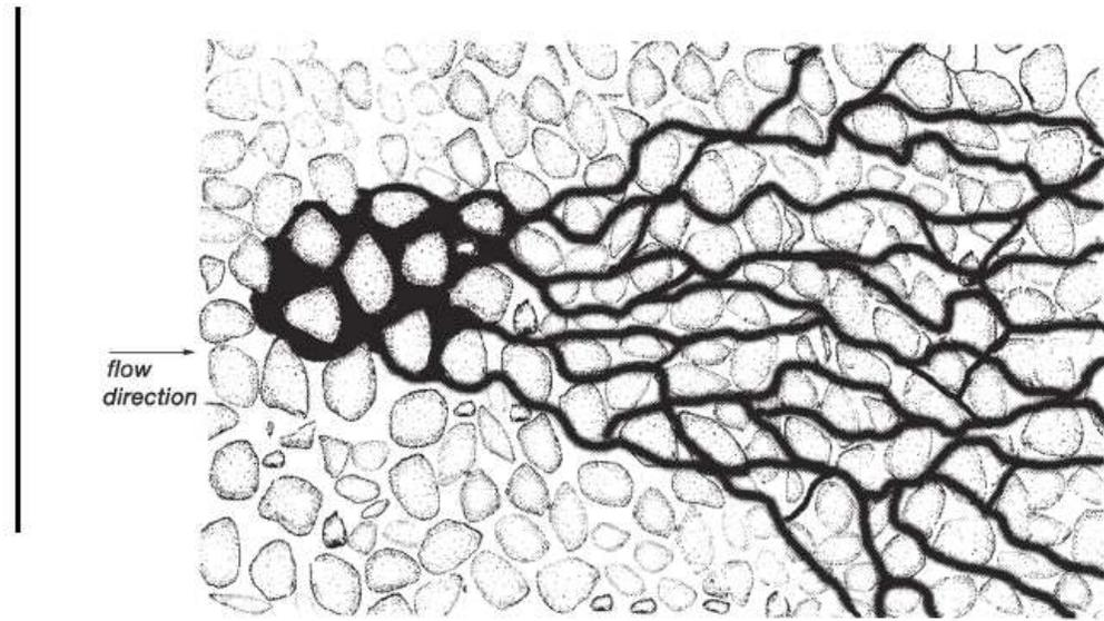
Fig.1 Contaminant transported in porous media
