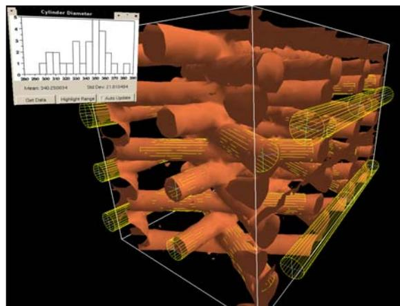
**Figure 34.** Cylinder measurement and analysis tool used on rendered objects derived from measured data taken from a tissue engineering scaffold.
