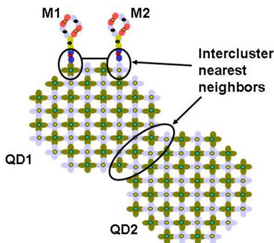
**Figure 30.** Illustration of intercluster nearest neighbors in a nano-system with four subsystems: two quantum dots (QD1 and QD2) and two conjugating molecules (M1 and M2).
