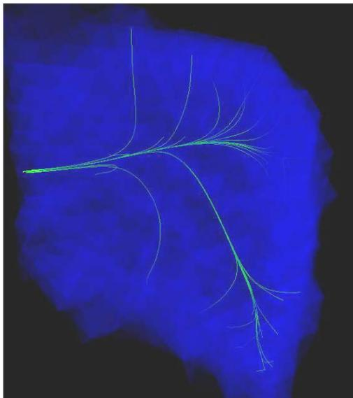
**Figure 42.** Curve-skeleton from an image file of a rock.
