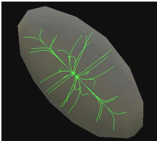
**Figure 43.** Curve-skeleton made from the divergence field on an ellipsoid.
