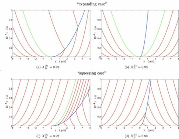
**Figure 26.** Trajectories of Kirkendall markers on the original interface (green) and at other initial positions (red). The blue trajectory is the position of the two-phase boundary.
