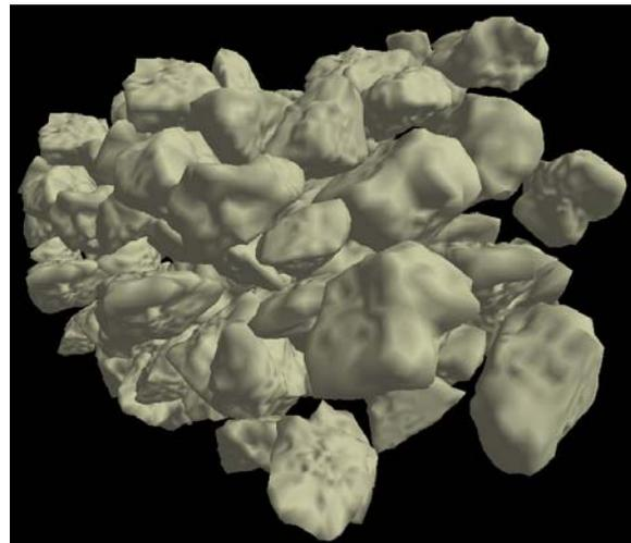
**Figure 37.** Snapshot from a computer simulation of a sheared suspension of cement particles. The cement particles shapes were obtained via X-Ray microtomography and are approximately 10-50 micrometers in size. These simulations play an important role in understanding how particle shape influences the rheological properties of suspensions.
