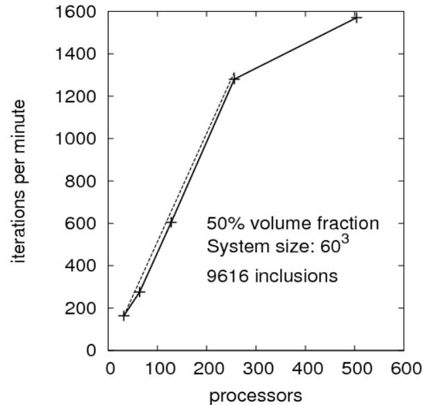
**Figure 31.** Scaling of new parallel algorithm on Columbia system. Above ~300 processors, the algorithm could handle a larger system size.
