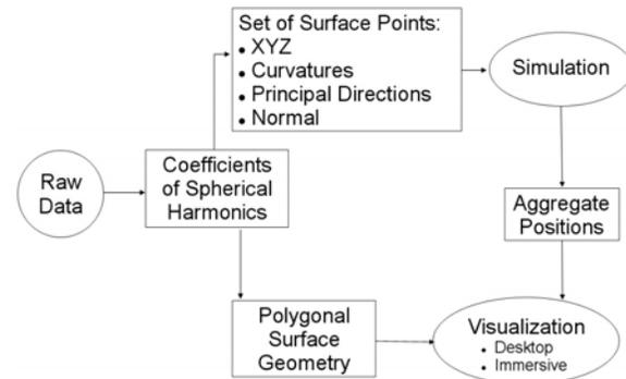
**Figure 35.** The raw data from the X-ray tomography of each aggregate is processed into one data set that is input into the simulation, and another data set that is used in the visualization.
