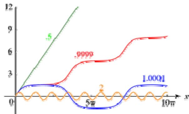
**Figure 46.** The Jacobian  $\text{am}(x, k)$  function for four values of the parameter  $k$ . These functions arise in the classical analysis of the dynamics of pendulums.
