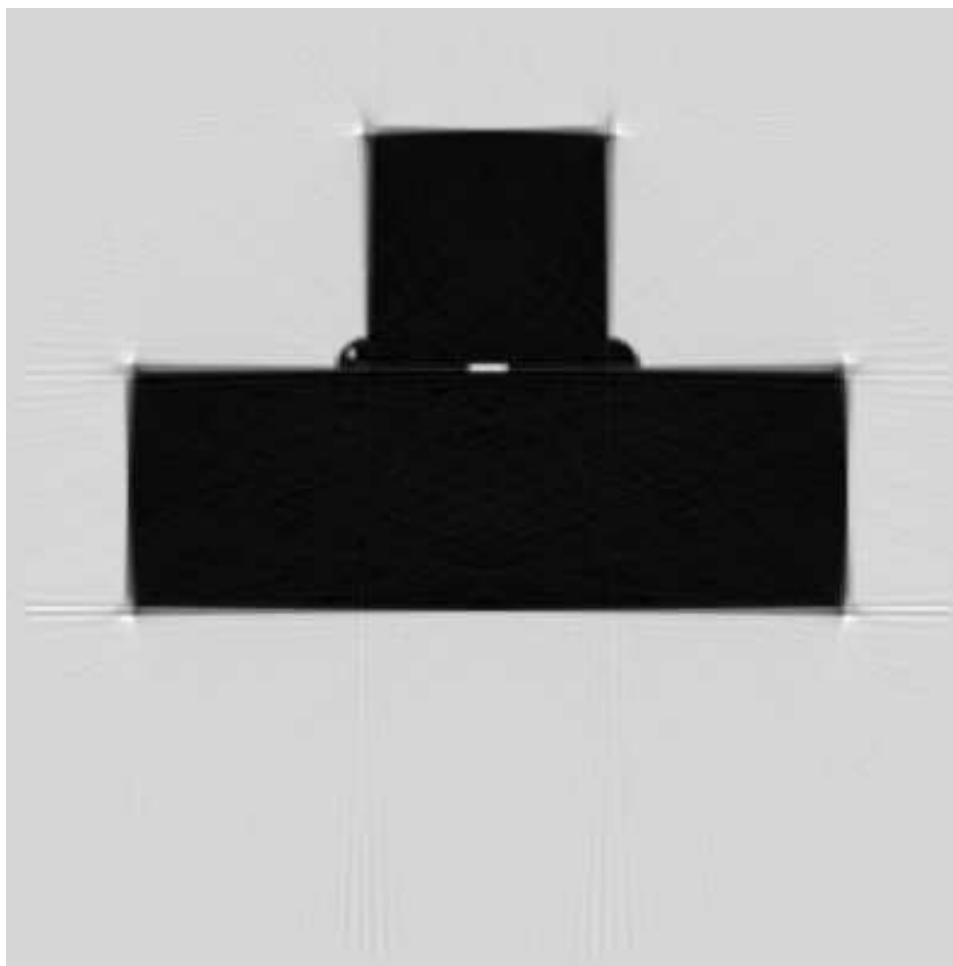
T-joint reconstruction from simulated data, 315 projections.
