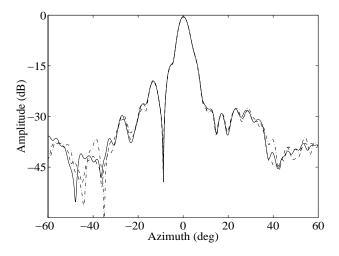
Fig. 5. H-plane far-field pattern of the dish (see section V-B). The solid line corresponds to the pattern without position errors. The dashed line shows the pattern computed from data on the plane  $z_0 + \lambda/4$ , also without position errors. The dotted line illustrates conjugate-gradient position error correction.
