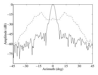
Fig. 2. H-plane far-field pattern of the radiometer. Probe position errors are given by eq (11). The solid line corresponds to the corrected pattern and to the actual pattern. The dashed line shows the result of ignoring the position errors.
