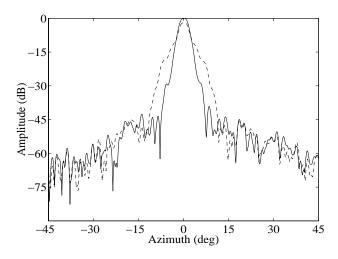
Fig. 1. H-plane far-field pattern of the radiometer. Probe position errors are given by eq (10). The solid line corresponds to the corrected pattern and to the actual pattern. The dashed line shows the result of ignoring the position errors.
