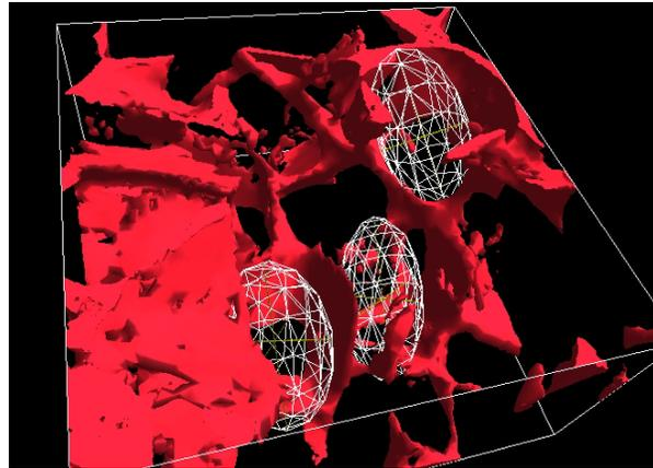
Figure 10. Ellipsoid measurement tool used on a scaffold.
