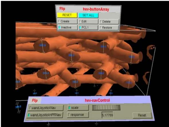
Figure 8. Scaffold cross sections with diameter measurements.
