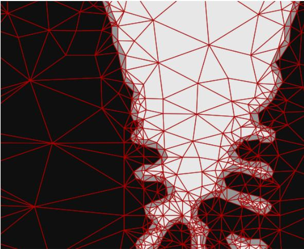
**Figure 19.** A portion of the microstructure, meshed with OOF2.
