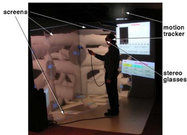
**Figure 7.** An IVE user making scaffold measurements.
