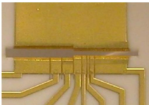
**Figure 15.** The multizone ion trap used in our experiments. The ions are trapped in the slot midway between the gold electrodes.
