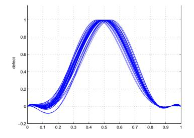
Plot of scaled defect vs  $\tau$  (ie.  $\delta(\tau)/\delta(\tau^*)$  vs  $\tau$ ) for each step required to solve a typical problem with SDC CRK6 and  $TOL = 10^{-6}$ .
